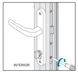
2 Turn Thumb Turn left or right to expose Cam Release Lever.
